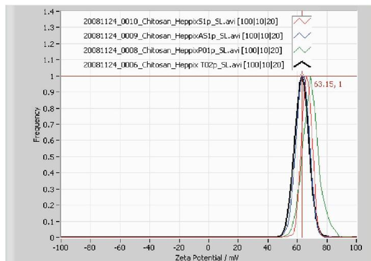
To make sure, that the results obtained with the ZetaView® are reasonable, titrations with charge calibrated anionic PVS solutions were performed in the Stabino®. The end point was 0 mV. It is known that the streaming potential at the starting point as well as the
